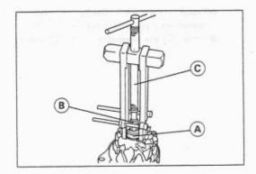
Press out the alternator rotor [A] from the alternator housing [B].
