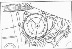
Detach the alternator [A] from the engine and then pull out the upper right mounting bolt [B].
