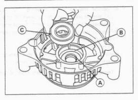
Install the bearing retainer with its mounting screws.
