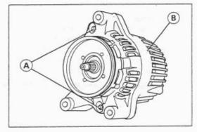
★If the alternator frame [A] is difficult to remove, use the crankcase splitting tool assembly [B].
